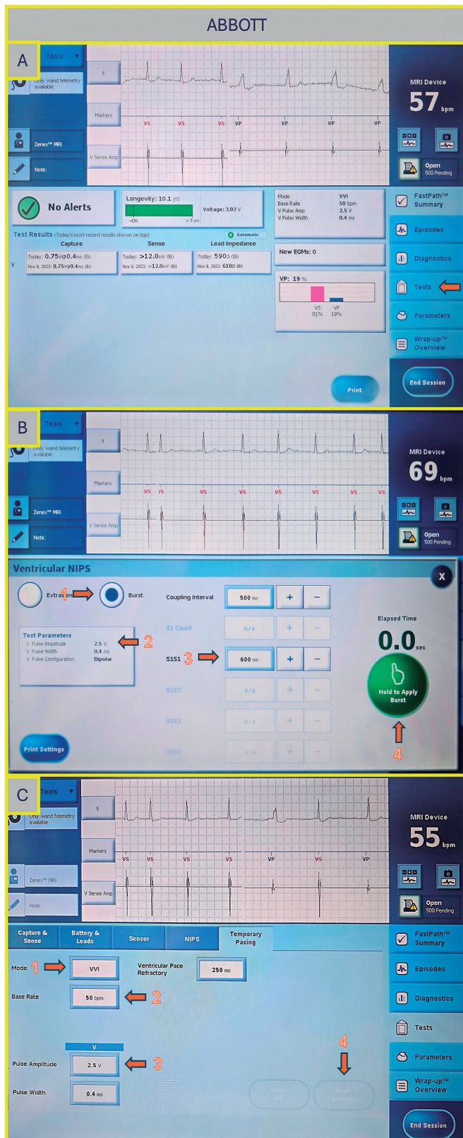
Figure 3. A: main screen of the Abbott/St. Jude console. Press “Test” to proceed to the electrophysiology study screen. B: ventricular NIPS screen. Select “Burst” (arrow 1), set the amplitude (arrow 2), adjust the S1–S1 interval (arrow 3), and press the green button to deliver pacing (arrow 4). C: temporary pacing screen. Select the pacing mode (arrow 1), desired rate (arrow 2), and pulse amplitude (arrow 3), then press the “Start Temporary” button (arrow 4).
