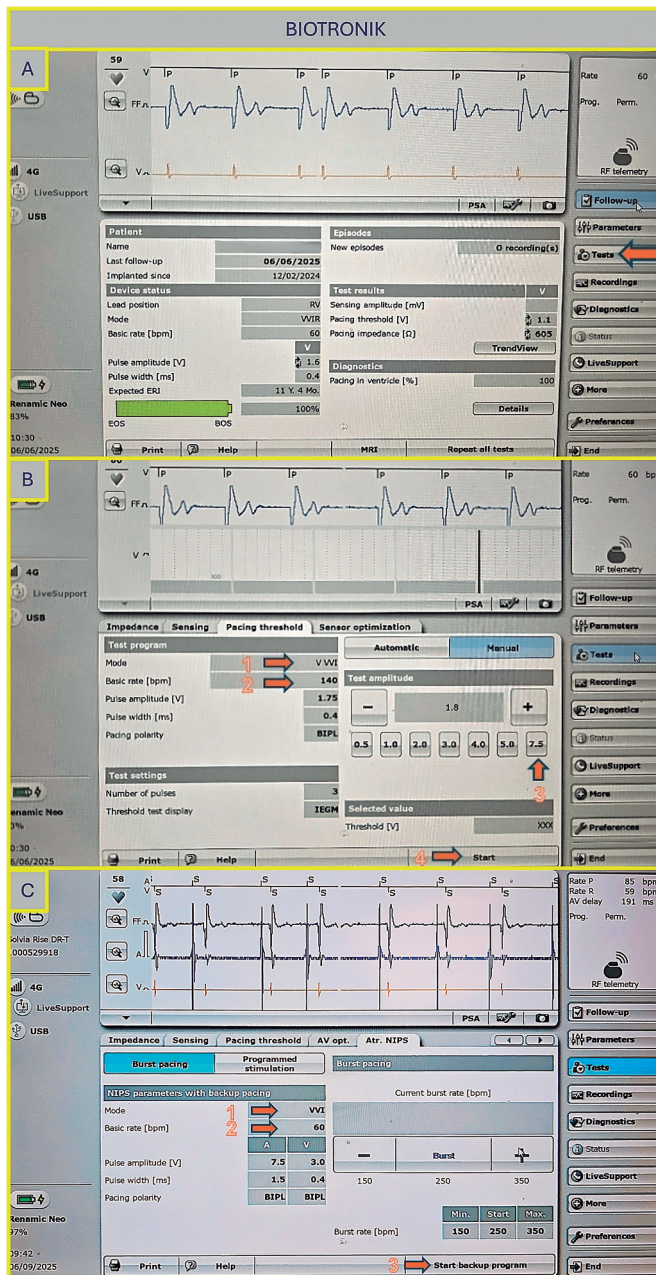
Figure 1. A: main screen of the Biotronik console. Select "Test" as indicated by the arrow to proceed to the pacing tests. B: to proceed to the pacing tests, select "Manual," then set the following parameters: pacing mode (arrow 1), basic rate (arrow 2), amplitude (arrow 3), and press "Start" to initiate pacing (arrow 4). C: configure the NIPS parameters by selecting VVI mode (arrow 1), setting the basic rate (arrow 2), and pressing "Start" to begin pacing (arrow 3). NIPS: Non-Invasive Programmed Stimulation.
