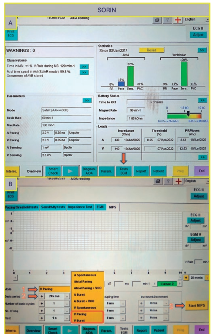
Figure 4. A: main screen of the Sorin console. Select "Tests EGM" (arrow) to access pacing options. B: "Tests EGM" screen. Select the pacing mode (arrow 1), the interval period (arrow 2), and then press the "Start NIPS" button (arrow 3).
