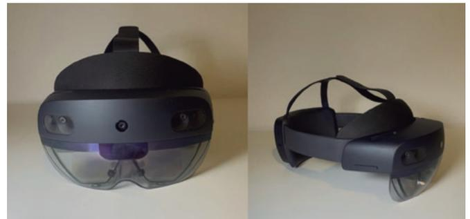
**Figure 1.** HoloLens extended mixed reality headset 2.
